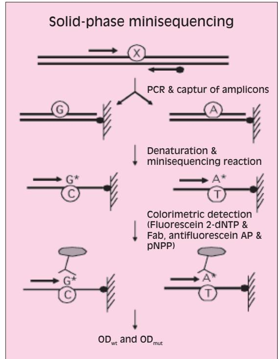
**Figure 1** - Principle of solid-phase minisequencing.
